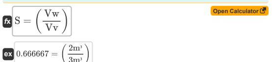
30) Volume of Voids given Degree of Saturation of Soil Sample
